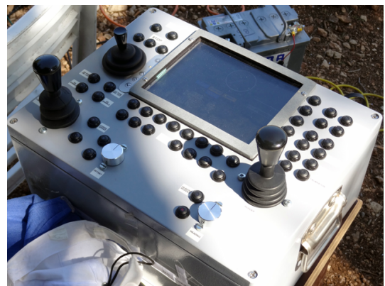
Fig. 4. Console-based Human Computer Interface
