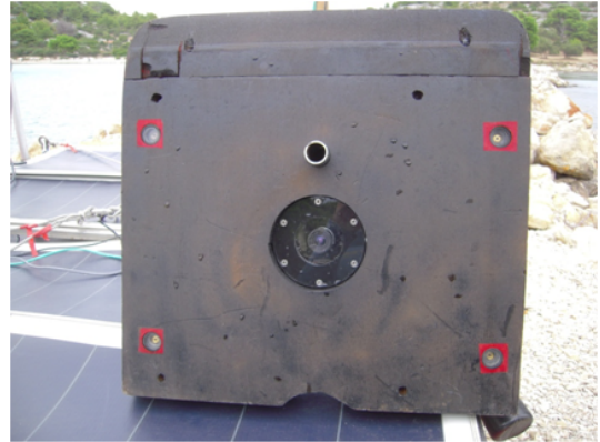
Fig. 2. The camera mounted together with the laser system
