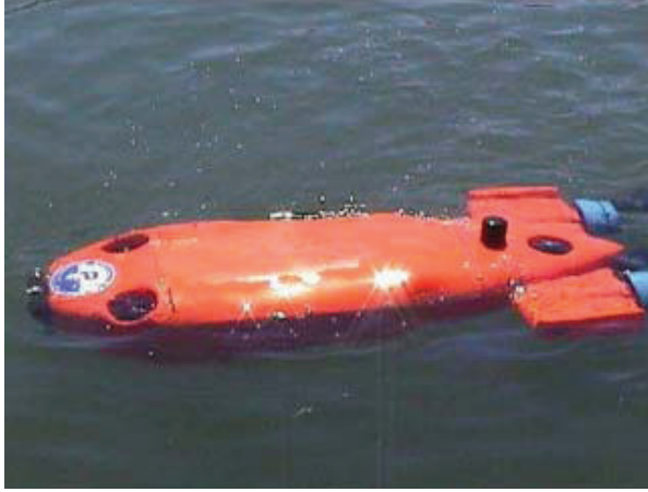
Fig. 3. CETUS II vehicle operated by SSC Pacific.
