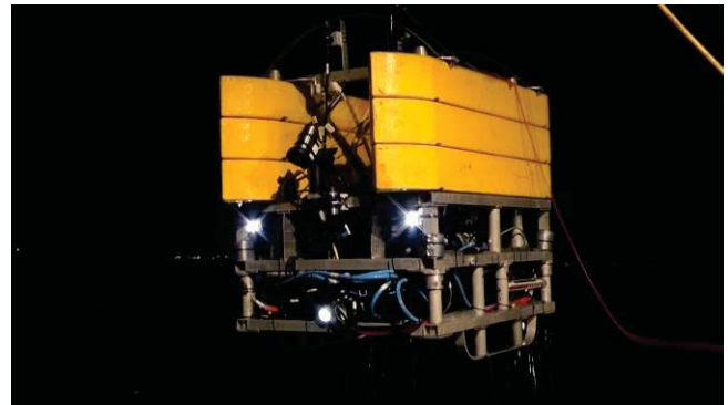
Fig. 1. Smart ROV LATIS, prototype platform with built-in OceanRINGS smart technologies.
