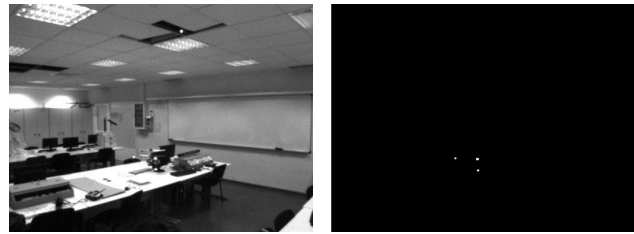
Fig. 6. The left image is the scene the left camera sees, it was taken without infrared filter. The right image is the same one taken with the infrared filter mounted on the camera and binarized. The three white points correspond to the helicopter leds.
