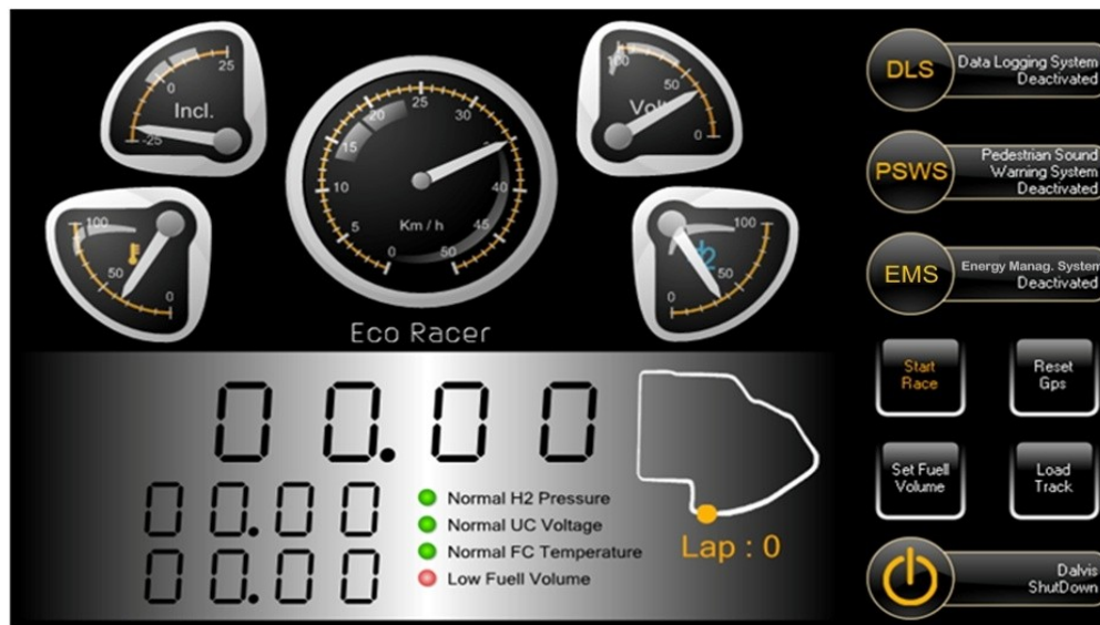
Figure 3: The driver's monitoring and control panel
