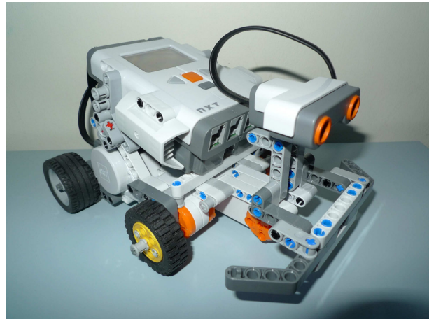
Fig. 2. Test platform: a cart build from Lego Mindstorms NXT constructor.
