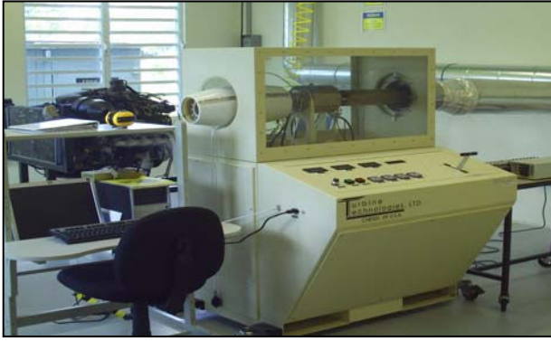
fig.1 SR-30 Gas turbine system
