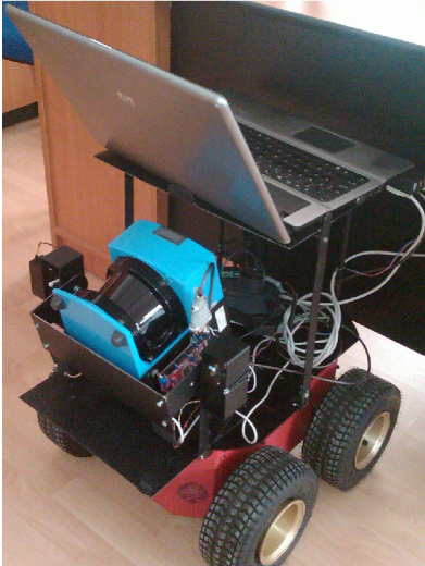
Fig. 3. The 3D scanner on the mobile robot platform.
