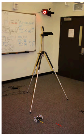
Fig. 8. The experimental environment. A camera in the VICON system, a Kinect, and a robot are shown.
