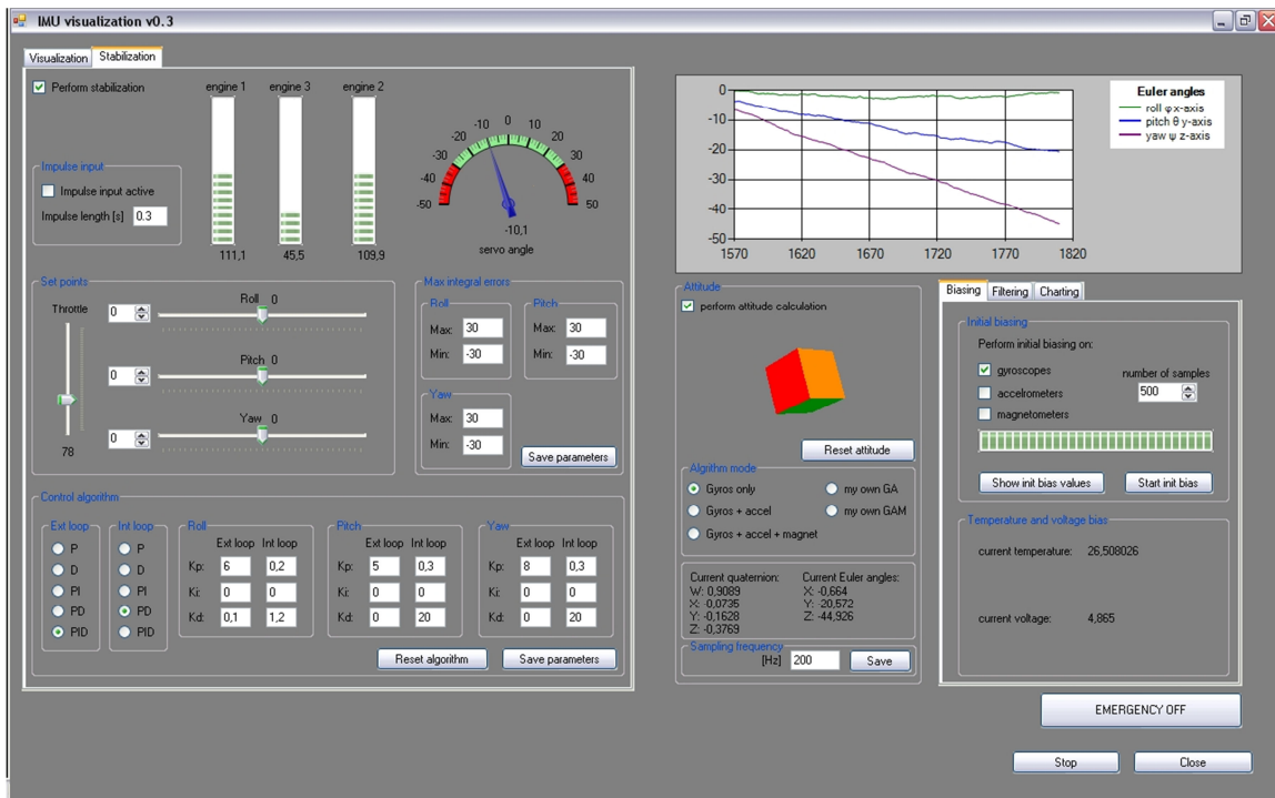
Figure 15. GCS application main window – stabilization and control tab
