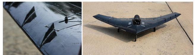
Figure 4. UCAV1303 fitted with a MVG.
