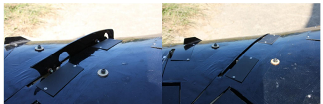
Figure 5. UCAV1303 fitted with a moving wing fence.
