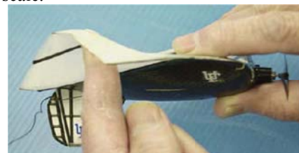
Figure 05. The chord-wise compliance of a flexible wing allows for passive-adaptive washout, increasing stability of the aircraft by Courtesy of Univ. of Florida
