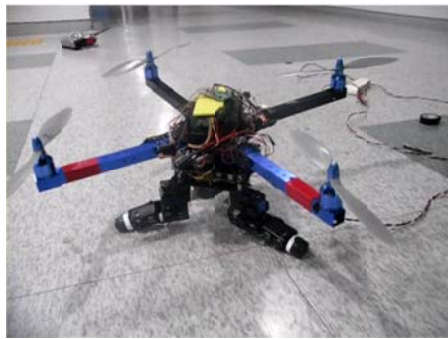
Figure 16 Multi-tentacle MAV system lands on flat surfaces.
