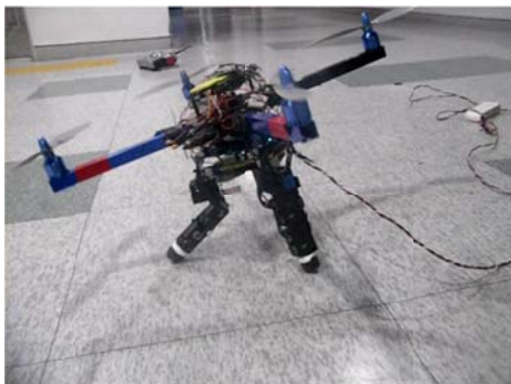
Figure 17 Multi-tentacle MAV system lands with one tentacle bend.
