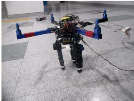
Figure 15 Multi-tentacle MAV system stands all tentacles stretched.
