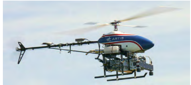
Fig. 1. Flight testbed for visual navigation. The picture shows DLR's 14kg helicopter ARTIS with a stereo camera and onboard computers [1].
