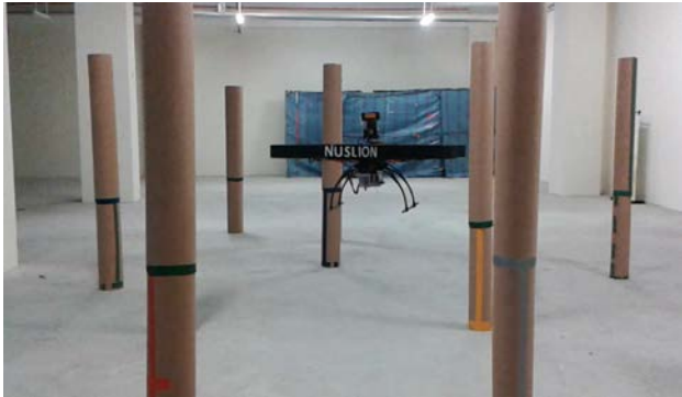
Fig. 9. Indoor test scenario for SLAM verification.
