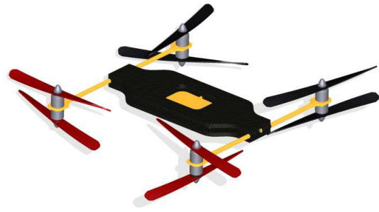
Fig. 3. A model of the morphing multicopter performing in a conventional horizontal body flight mode.
