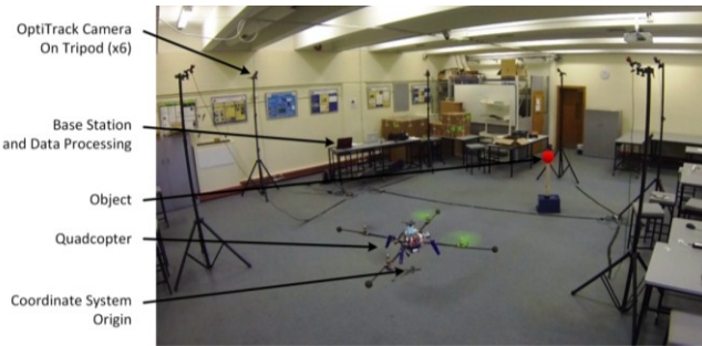
Fig. 6. External camera system experimental setup.
