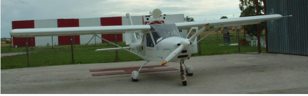
Figure 4. FLARE with radar/optical sensors installed on top of the wing
