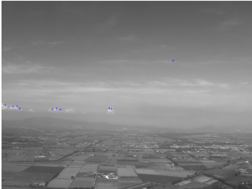
Figure 11. Single frame detections obtained using morphological filtering and global thresholding, without local analysis of regions of interest (test case 1)
