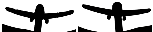
Fig. 6: Masks developed for robust homography estimation. The areas colored in black are not considered for the search of strong corners.
