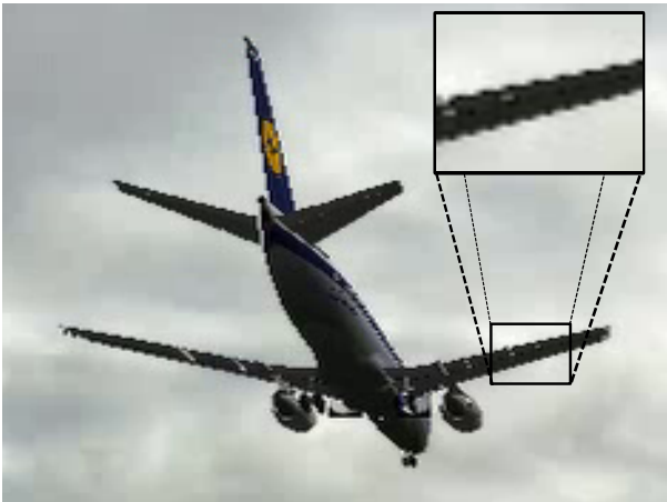
Fig. 7: Close view of a simulated intruder. Edges appear interpolated with the background increasing the realistic appearance of the intruder.
