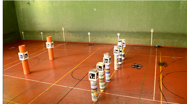
Fig. 1. Experimental flight of the basic instance of the framework, which is characterized by swarm behavior, using 5 AR Drones. The row of columns represents a virtual wall with a single 1.5 m opening in the middle. In order to simplify the localization problems the columns are marked using ArUco visual markers [2]. In this flight the mission of the swarm is to cross from one side to the other, each swarm agent also has to avoid collision with the columns or the other drones. This test was designed to showcase the capabilities of the basic instance of the framework.
