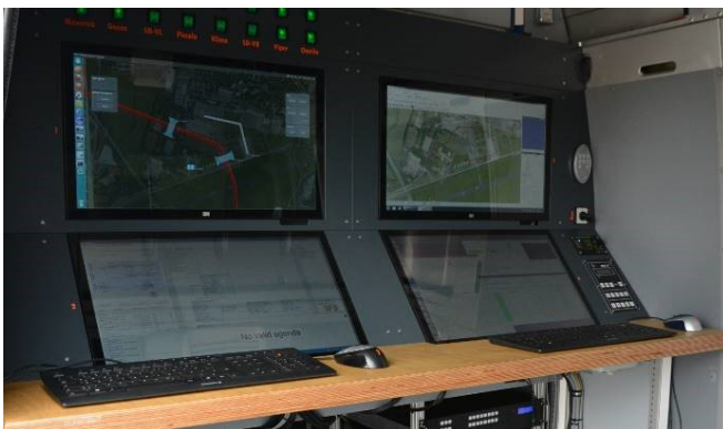
Figure 10. GCS with the operator workplace (left) and flight-test environment (right).
