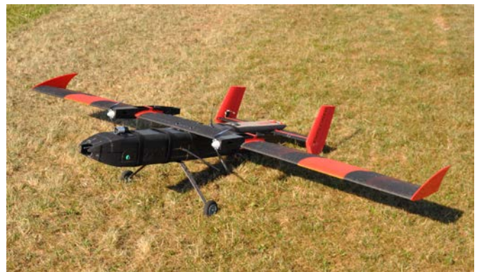
Figure 11. UAV demonstrator Explorer as aircraft platform for flight-testing
