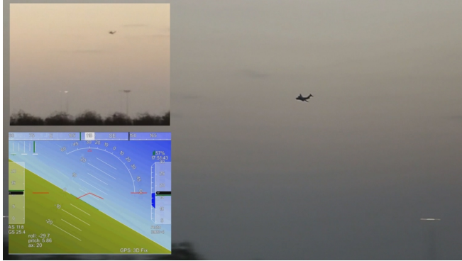
Fig. 6. Upper figure: a picture of the UAV model used. Lower figure: UAV during autonomous flight at 11 m/s, during a flight test aimed at validating the possibility of dynamically rerouting the UAV.
