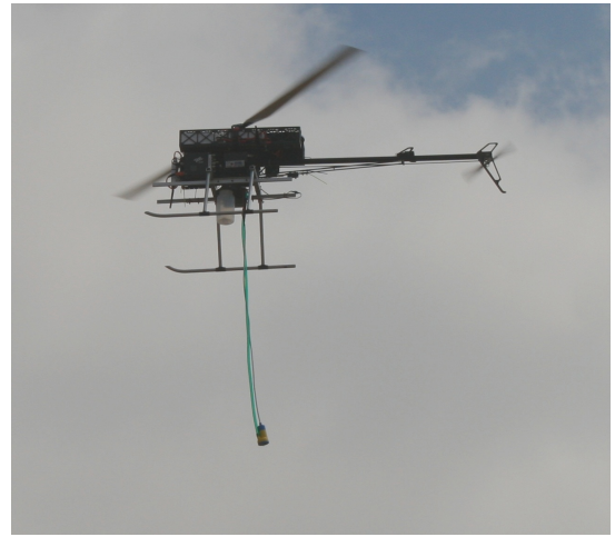
Fig. 5. UAV with water sampling mechanism in flight
