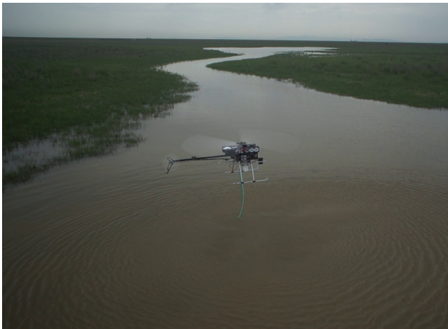
Fig. 7. Automatic water sampling application in national park
