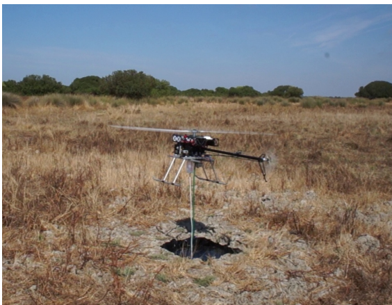
Fig. 1. Automatic water sampling demonstration in national park
