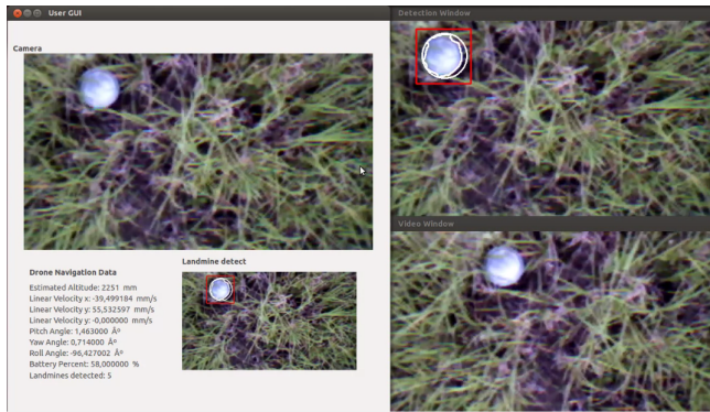
Fig. 5. GUI components: (upper-left) image received from the bottom camera of the AR.drone, (lower-left) navigation data and output-image with the detected landmine-like object, (lower-right) live video received from the AR.drone.
