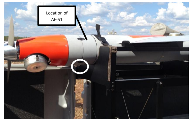
Pic. 4. Photo showing the position of the inlet tube for the AE-51 (circled in white). The inlet stuck out of the bottom of the fuselage through one of the holes where an extra screw was used. The inlet only extended 1.3 cm from the fuselage to minimize the effect of wind on the inlet tube shape and orientation.
