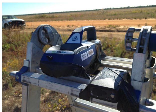
Pic. 2. Instrumentation setup for small plot burns (S5-S3). Both the DustTrak (left) and the microAeth (right) were collecting smoke samples for all three small burns. The ladder was 1.3 meters high.
