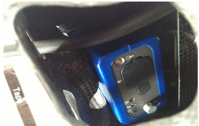
Pic. 3. Photo showing the placement of the microAeth (AE-51) in the fuselage compartment of the Boeing ScanEagle. The AE-51 was positioned in the back of the fuselage and held in place by Velcro. Weight and balance adjustments were made after the integration.
