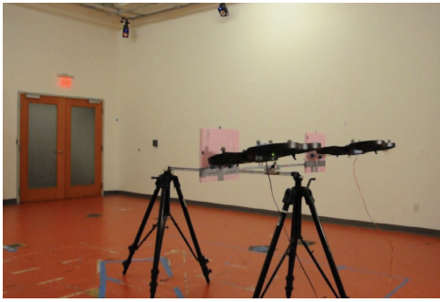
Fig. 8: Testbed platform for aerial manipulation between two quadrotors.
