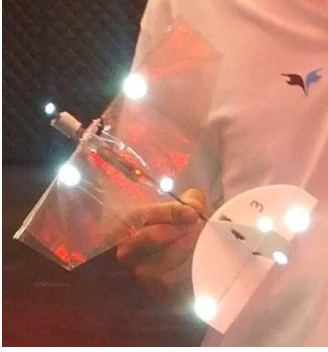
Fig. 2. Markers' positions on the DelFly, respectively placed at the nose, trailing edge of the wing, wing stiffeners' intersection with leading edge rod, fixed horizontal and vertical stabilizers, elevator and rudder.
