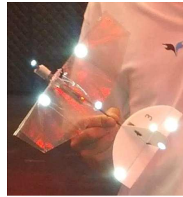
Fig. 1. The DelFly FWMAV configuration and reflective markers' positions.
