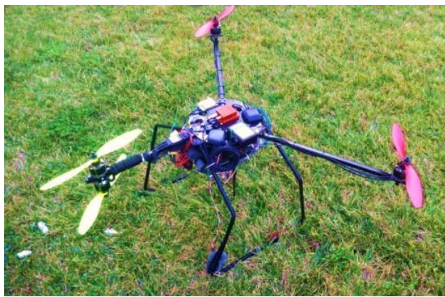
Figure 16 One of the first multicopter prototypes of TURAC is used when developing autopilot
