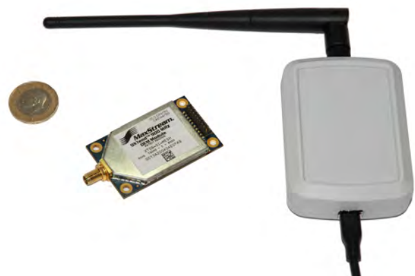
Fig. 6: Xtend 900Mhz transponders for hardware emulation of ADS-B
