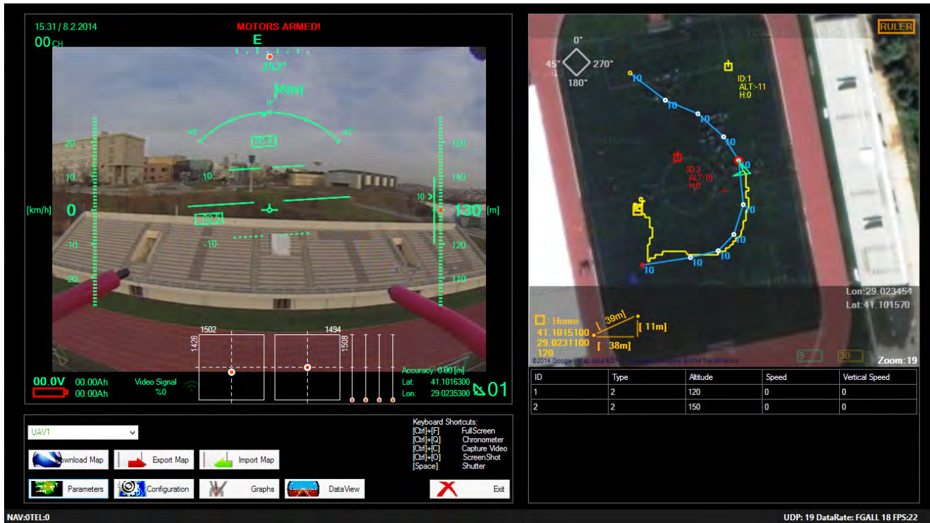
Fig. 2: Graphical User Interface screen on the ground station during flight test
