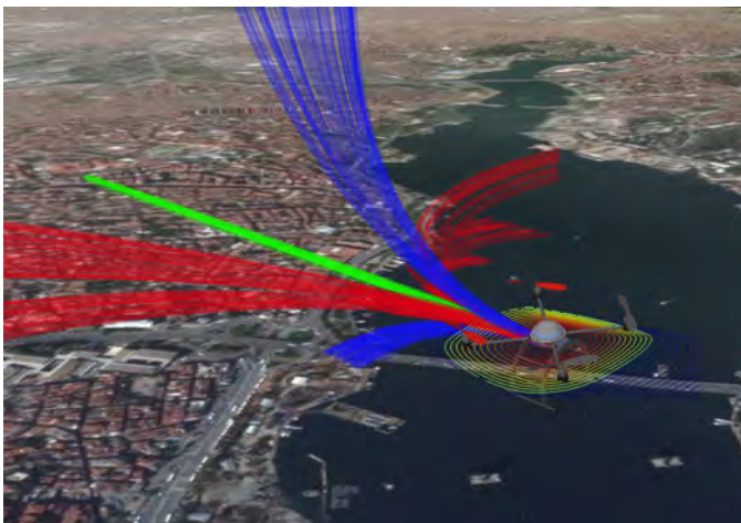
Fig. 12: Running of sense-and-avoid algorithm with probabilistic modal maneuver search
