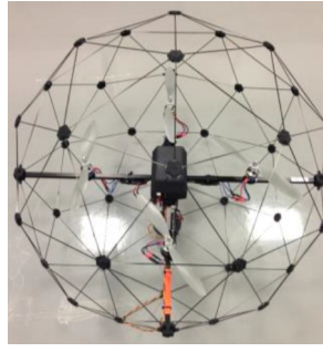
Figure 2. QUANSER's Qball-X4 UAV
