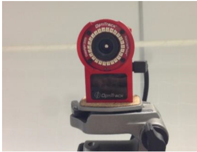
Figure 4. Optitrack camera used as a localization system.
