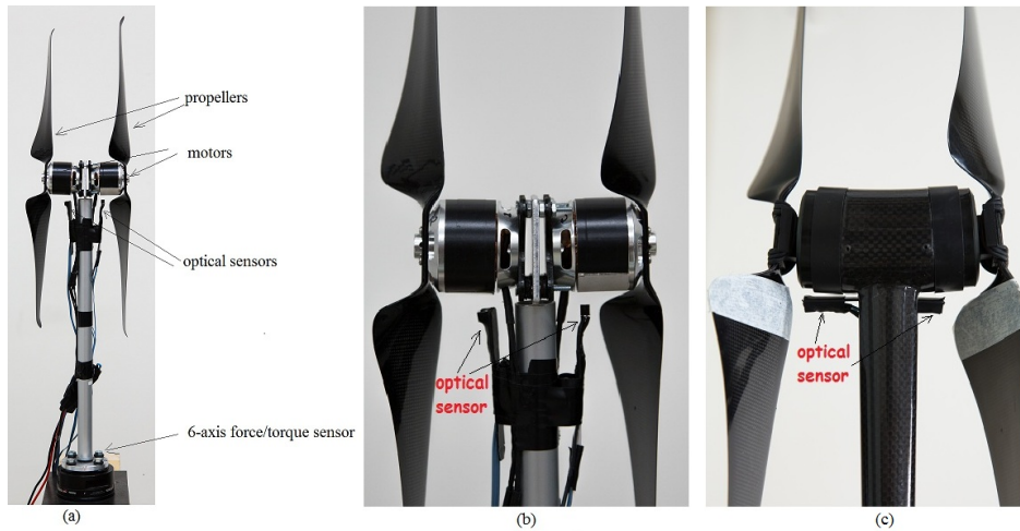
Fig. 2. (a) thruster identification test stand; (b) optical sensor mounted on the test stand; (c) optical sensor mounted on X8
