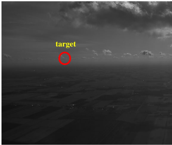
Figure 4. Frame from video stream VS1 with distant target aircraft under cloudy conditions and medium background clutter (distance to target: 0.94 km / 3084 ft).
