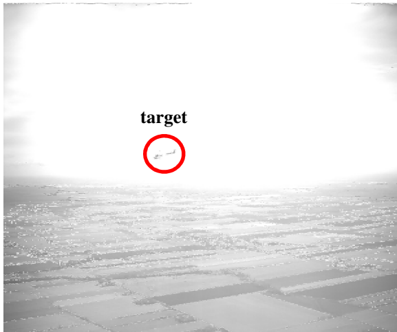
Figure 5. Frame from video stream VS2 with close range target aircraft under glare conditions and medium background clutter (distance to target: 0.14 km / 446 ft).
