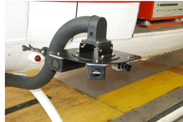
Figure 3. Camera mount designed to hold the 3 Prosilica Imagers on the Bell 205 aircraft.
