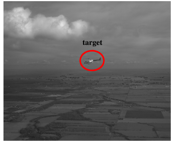
Figure 6. Frame from video stream VS3 with close range target aircraft under cloudy conditions and high background clutter (distance to target: 0.24 km / 782 ft).
