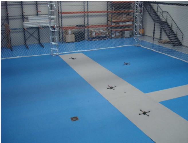
Fig. 8. Multi-UAV testbed placed in the CATEC facilities.
