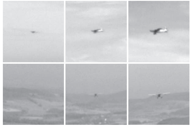
Fig. 7. Comparison of aircraft patches (100 x 100 pixel) from a Pilatus PC-6 at different distances: 3.0 km, 1.5 km and 1.0 km. The top row shows a crossing from the right and the bottom row a head-on scenario.
