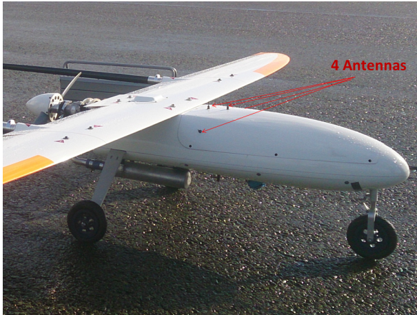
Fig. 5. Broadband payload data link: 4 small antennas are integrated in the Penguin B UAV fuselage.
