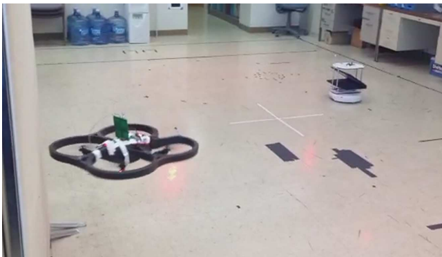
Fig. 15. Real time experimental application for the case of a moving source. The source is moving in a circle, and the quadrotor is flying to four navigation points located around the source region.
