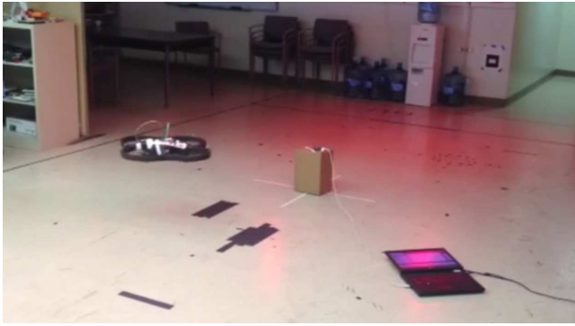
Fig. 13. Real time experimental application for the case of a static source. The quadrotor can be seen flying around the source.
