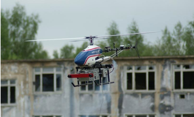
Figure 1. The unmanned helicopter ARTIS equipped with realtime 3D obstacle detection based on stereo vision.
