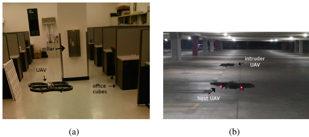
Fig. 6: Two experiment situations: (a) avoid a static obstacle in an office; (b) avoid another ARDrone in a parking structure.
