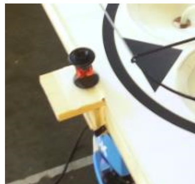
Fig. 2. Details of the installed reflector to track the position of UGV in outdoor GPS-denied environment
