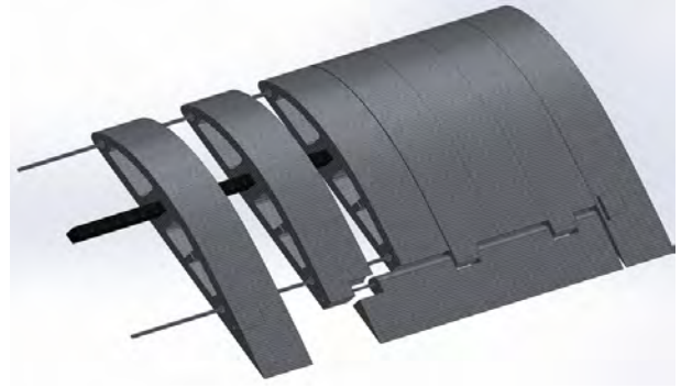
Fig. 3. This is an inside view of the 3D printed plane wing displaying the segmented sections utilized for 3D printing efficiency, as well as allowing for ease of substituting sections with new embedded sensors
