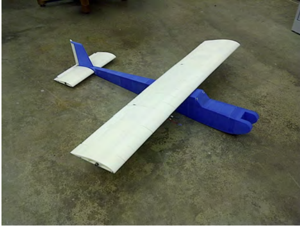
Fig. 1. Fully 3D printed plane prototype
