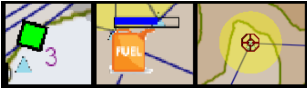
Fig. 5. (a) UAV with low navigation, high health monitoring, and high state/autopilot autonomy. (b) Icon of fuel station used for UAV refueling. (c) Search target (red) and search zone (yellow)
