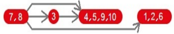
Fig. 2. The graph delivered by Tarjan's algorithm when applied to the graph (U, \tilde{\Phi}) from Figure 1. Its vertices represent strongly connected components in the original graph.
